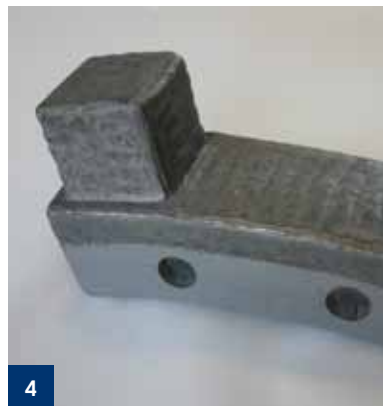
1. Chromium carbide on 3/4 Hardox 450 as bottom plate for longwall face conveyor pan line sections
