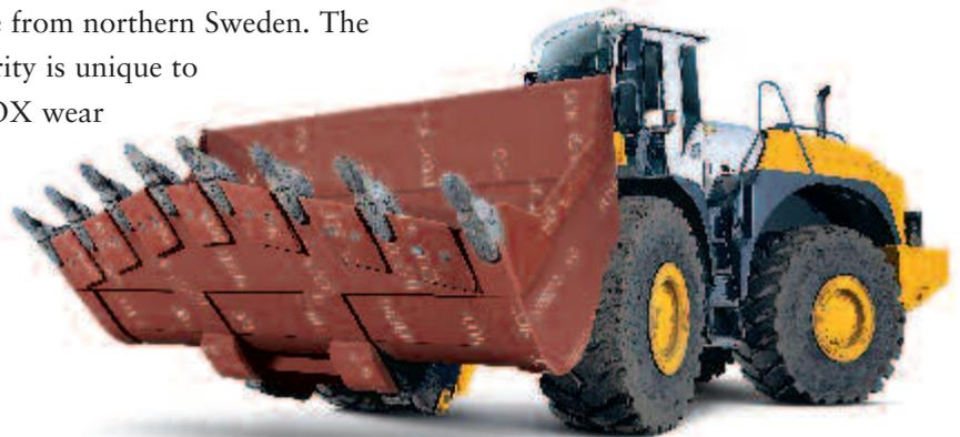
The various hardness grades of HARDOX steel have optimum locations in the bucket. HARDOX 450, for example, is very well suited for the body of the bucket, while HARDOX 500 is appropriate for the cutting edge. HARDOX HiTuf is eminently well suited for very thick cutting edges of large buckets.
