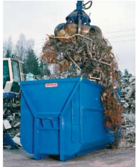
Advertising sign. A container made of HARDOX wear steel has a long useful life and resists wear very effectively. The smooth sides of the container can serve as an advertising sign for the company it represents.
